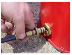
7. Free in-line fuel valve by pushing with a stick
