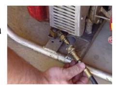
10. Squeeze fuel line bulb. Observe gas being forced up sight tube, then STOP squeezing
