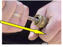
8. Check for fuel flow while holding valve open with stick. Squeeze in-line primer pump bulb. No fuel is #1 problem cause.
